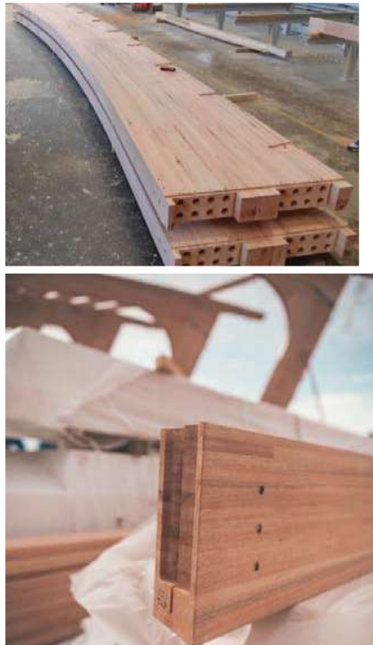
Figure 10: CNC machining in the beams and purlins
